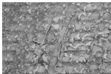
Fig. 46 Mounted TC 7 and 10 on ablator surface
