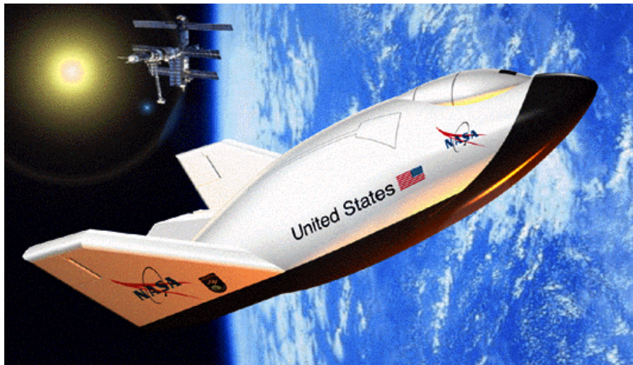
Fig. 4 X-38 NASA technology demonstrator for the ISS CRV © NASA
