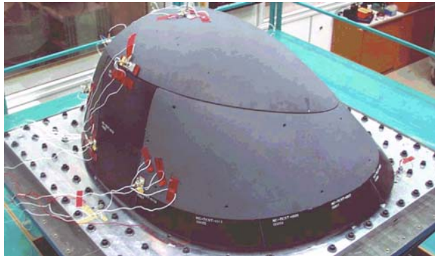
Fig. 12 Vibration test set-up of the X-38 nose qualification model (©IABG)
